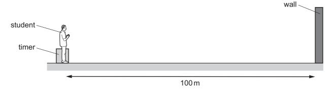
An electronic timer detects the echo of the sound 0.60s after it is made.
