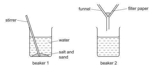
The contents of beaker 1 are stirred and then poured into the funnel above beaker 2.
