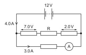
What is the p.d. across resistor R, and what is the current in resistor R?
