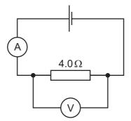
Which pair of meter readings in the table is possible?
