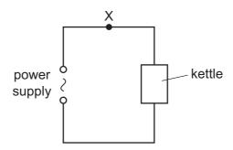
If too much current flows, a component connected at X automatically disconnects the power supply.
