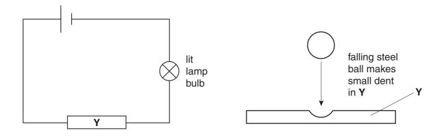
The tests show that Y conducts electricity and is hard.
