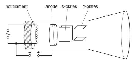
From which component do the cathode rays start?
