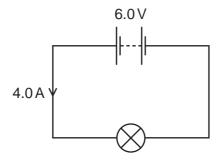
A current of 4.0 A flows in the circuit for 20 s.
