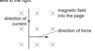
In which direction is the force when the current direction is reversed?
