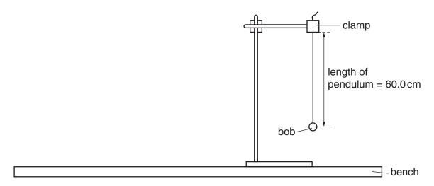
Retort stands of 60 cm or less in height may be used if the retort stand is reversed so that the pendulum hangs below the level of the bench. The base of the stand would need to be secured with a G-clamp and/or a heavy weight. Supervisors would need to warn candidates of the difference between this diagram and the set-up of their experiments.
