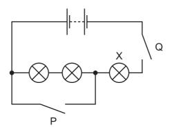
Which of the switches must be closed so that **only** lamp X is lit?
