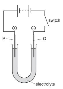
When the switch is closed, the solution around electrode P turns orange because a halogen is formed.
