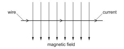
The magnetic field causes a force on the wire.
