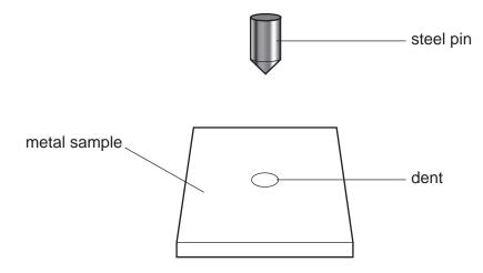
The depth of the dent produced is measured on a scale of 0 to 100.
