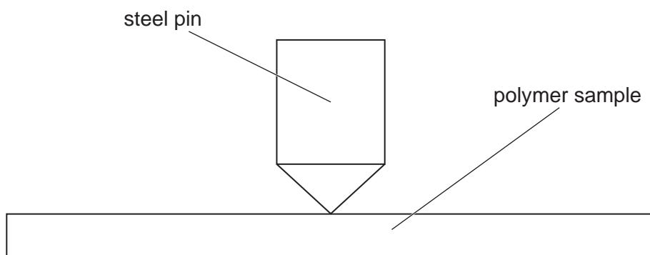
When a force is applied to the pin it sinks into the polymer sample. The diameter of the dent made in the polymer sample is measured.
