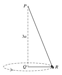
A light inextensible string of length 4a has one end fixed at a point P and the other end fixed at a point Q, which is vertically below P and at a distance 3a from P. A small smooth ring R of mass m is threaded on the string. R moves in a horizontal circle with centre Q and with the string taut (see diagram).
