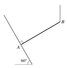
The rod rests with A on a rough plane that makes an angle of  $60^{\circ}$  to the horizontal. A string is attached to B and the rod is in equilibrium in the vertical plane containing the line of greatest slope of the plane, with the string vertical and AB perpendicular to the plane (see diagram). Find the magnitude of the frictional force at A and the tension in the string.
