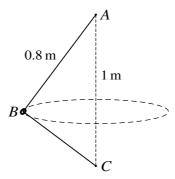
A light inextensible string of length 1.4 m has its ends attached to two points A and C, where A is 1 m vertically above C. A smooth bead B of mass 0.2 kg is threaded on the string and rotates in a horizontal circle with the string taut. The distance BA is 0.8 m (see diagram). Find
